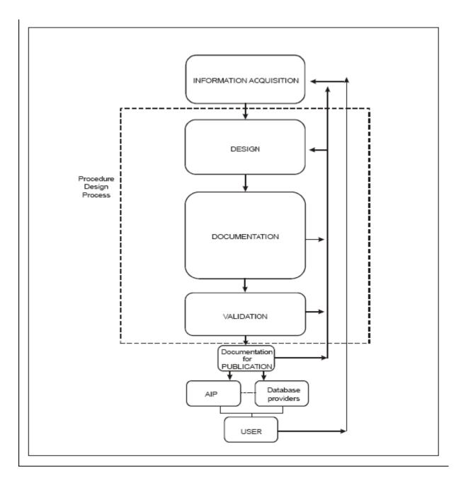
Instrument Flight Procedure Design Process
