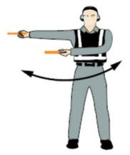
Extend arm horizontally at a 90-degree angle to right side of body. Move other arm in same direction in a sweeping motion.
