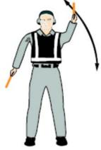
Point right arm with wand down and bring left arm from overhead vertical position to horizontal forward position, repeating left-arm movement.
