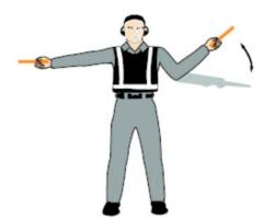
With right arm and wand extended at a 90-degree angle to body, make "come ahead" signal with left hand. The rate of signal motion indicates to pilot the rate of aircraft turn.
