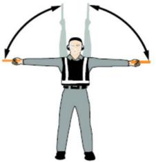
Fully extend arms and wands at a 90-degree angle to sides and, with palms turned up, move hands upwards. Speed of movement indicates rate of ascent.
