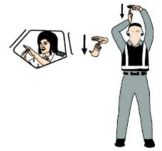
Hold arms fully extended above head with finger tips of right hand touching open horizontal palm of left hand (forming a "T"); then move right hand away from the left.
