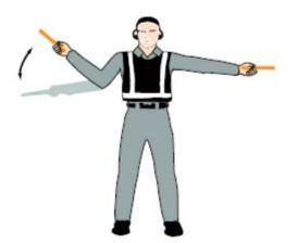
With left arm and wand extended at a 90-degree angle to body, make "come ahead" signal with right hand. The rate of signal motion indicates to pilot the rate of aircraft turn.
