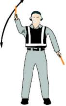
Point left arm with wand down and bring right arm from overhead vertical position to horizontal forward position, repeating right-arm movement.
