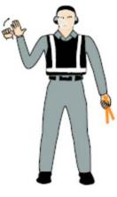
Raise hand just above shoulder height with hand closed in a fist. Ensuring eye contact with flight crew, open palm. **Do not** move until receipt of "thumbs up" acknowledgement from flight crew.
