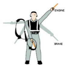
Move right-hand wand in a "fanning" motion from shoulder to knee, while at the same time pointing with left-hand wand to area of fire.
