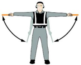
Fully extend arms and wands at a 90-degree angle to sides and, with palms turned down, move hands downwards. Speed of movement indicates rate of descent.
