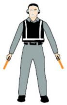
Fully extend arms and wands downwards at a 45-degree angle to sides. Hold position until aircraft is clear for next manoeuvre.
