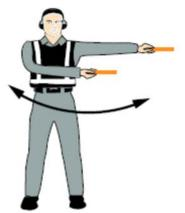
Extend arm horizontally at a 90-degree angle to left side of body. Move other arm in same direction in a sweepingmotion.
