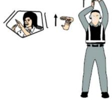
Hold arms fully extended above head; open left hand horizontally and move finger tips of right hand into and touch open palm of left hand (forming a "T"). At night, illuminated wands can also be used to form the "T" above head.
