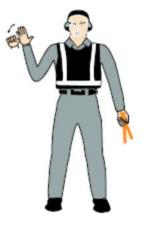
Raise hand just above shoulder height with open palm. Ensuring eye contact with flight crew, close hand into a fist. **Do not** move until receipt of "thumbs up" acknowledgement from flight crew.
