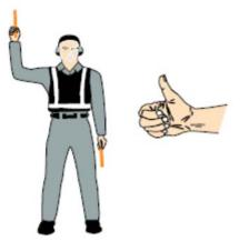
Raise right arm to head level with wand pointing up or display hand with "thumbs up"; left arm remains at side by knee.
