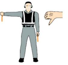
Hold right arm straight out at 90 degrees from shoulder and point wand down to ground or display hand with "thumbs down"; left hand remains at side by knee.
